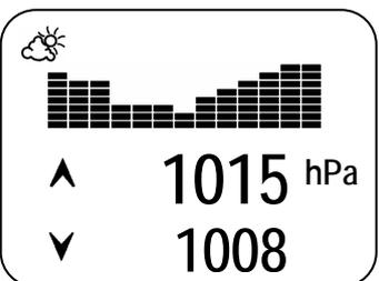
**Barometer display with max and min pressure**
