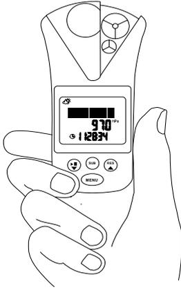
The Windwatch *PRO* is designed to precisely measure the wind speed regardless of the prevailing air density. In order to obtain optimal results, the instrument should be held vertically into the wind with an outstretched arm. To insure the greatest accuracy, measurements should be taken where there are minimal obstructions upwind of your position that might cause turbulence.
