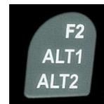
Altitude display **Alt1** indicates always the absolute pressure altitude above sea level. After switch-on the altimeter ALT1 is automatically adjusted to GPS altitude by the instrument. After switch-on the display is flashing until the GPS-receiver has calculated a precise altitude for adjustment.
