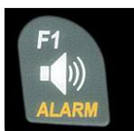
During flight it is possible to switch-on or to switch-off each alarm by long pressure on **key Alarm** → **Sensor x**, and on key F1.
