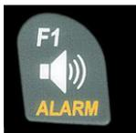
During flight the stall alarm can be switched-on or switched-off by prolonged pressure on the **key Alarm** → Stall by use of the keys F1 / F2.
