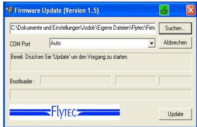
Now connect the USB cable with the instrument. Afterwards you can set the interface in the field Com Port, or if it is unknown to you, set to **Auto** and have thereby an automatic search prompted. The virtual COM interface should be positioned between 1 and 8. Above this value the Flasher can no longer recognise the interface.
