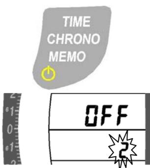
To switch the instrument *OFF* press and hold the *TIME/CHRONO/MEMO* Key for about **seven seconds**.
