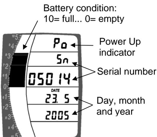
The Startup Screen shows the serial number, the battery condition and the date. The analog scale on the left shows the battery charge.
