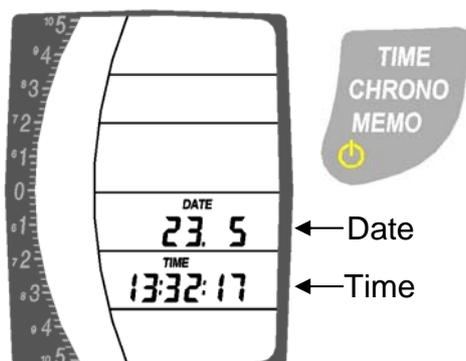
The date and time are displayed when the instrument is off.
