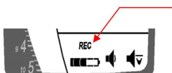
For a flight to be recorded in the logbook, an altitude difference of more than +/-100 feet (30 meters) and a flight time of more than two minutes must be achieved (this prevents wasted flights in the logbook). The **flight acceptance** on a 6000 will be confirmed with the **REC** Indicator.
