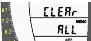
While in MEMO display, use a 3-second press on the MEMO Key to bring the instrument into Memory Set-Mode. The display will now show CLEAR ALL, which allows you to delete all flights in the logbook. To confirm, press the ALT1/ALT2 Key for at least three seconds until you hear the confirmation tone.
