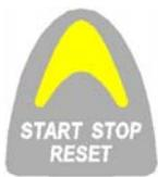
When in TIME or CHRONO display, use a short press on the START/STOP/RESET Key (the up arrow) to start and stop the stopwatch. There are instances where the stopwatch is not displayed depending on which mode the instrument is in – however it will continue to run until it is stopped (or the instrument is switched off). A three-second press on the START/STOP/RESET Key will reset the stopwatch to zero.
