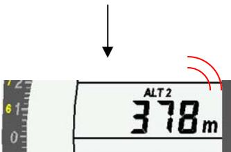
In *ALT2* Set-Mode you can set a reference altitude (for example, the relative altitude to a goal or waypoint). In order to do this *ALT2* must be set to relative altitude (see Option 2 below
