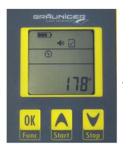
The SensBox points in longitudinal axis to 178°
