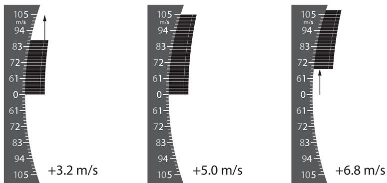
A second, narrow bar just to the right of the wide bar on the graphic vario represents your average vertical speed by indicating the current value of the numeric vario (see next section).
