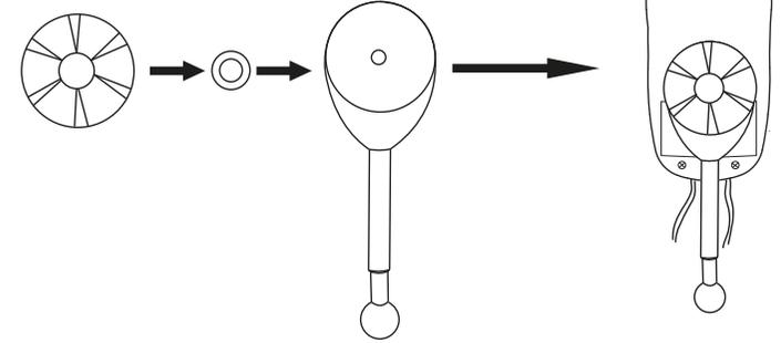
Fix mount and safety lanyard to the control bar
