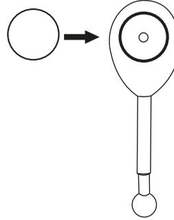
Back: Add washer and screw to the disc and attach to the back of the Element
